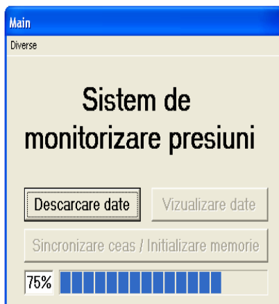
Fig. 20. Showing the data transfer initiation between the computer and the acquisition system
