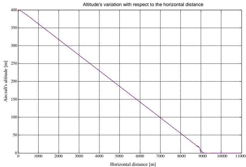
Fig.13 The time variation of the flight altitude for the entire landing process
