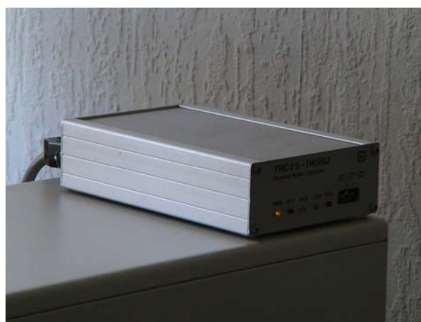
Fig.5. The modem of 'R1' has two firmware (software installed within its EPROM). We configured one of them, TAPR 1.1.8 , to work in KISS mode
