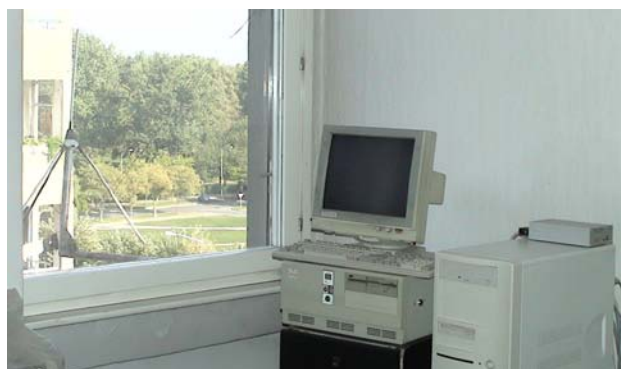
Fig.4. Node 'R1' elements: Outdoor antenna (left), control computer (middle), modem (top right), VHF radio station (behind the computer)
