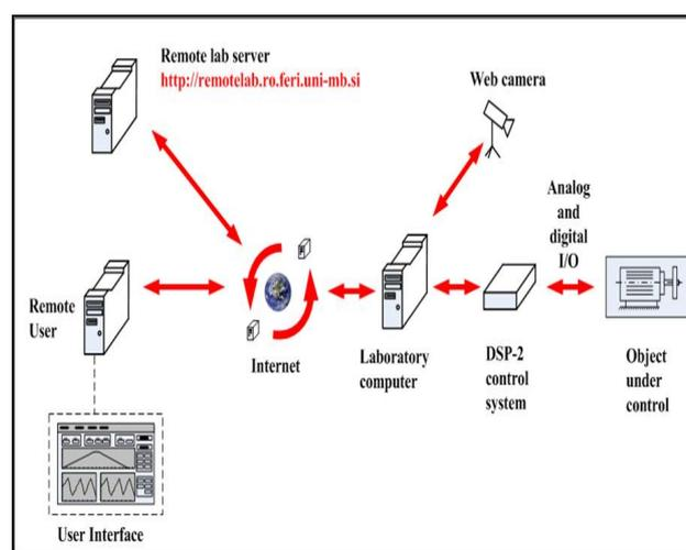
Fig. 1 Architecture of the Remote Laboratory
