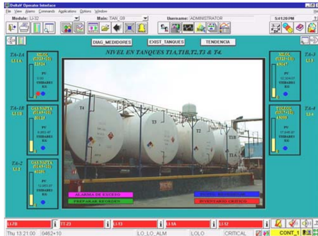
Fig. 8 The Operator Interface for the system.
