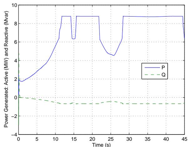
Figure 3: Generated active and reactive power
