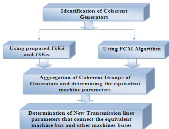
Fig. 2 The block diagram of the main steps of the construction of power system dynamic equivalent
