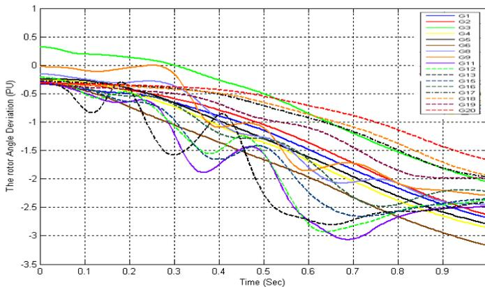
Fig. 9 the time response for 118-Bus IEEE system machines after clearing fault
