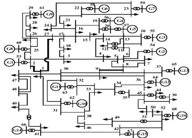
Fig. 4 Single line diagram of 68 bus system
