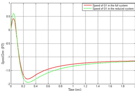
Fig. 6 speed deviation of generator no. 1 in the original system and in the reduced system
