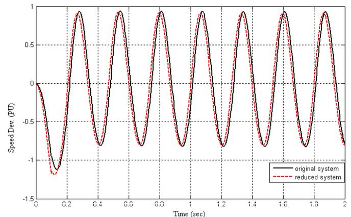
Fig. 5 Speed deviation of generator No. 6 in the original system and in the reduced system
