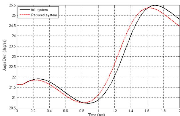
Fig. 11 speed deviation of generator no. 9 in the original system and in the reduced system
