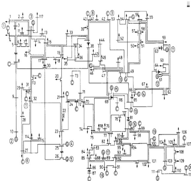
Fig. 8 Single line diagram of 20-machines IEEE-test system
