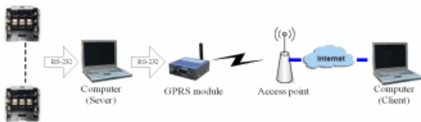
Fig. 6. A wireless network structure between client computer and controlled PM contactor.
