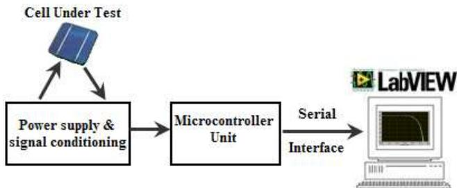
Figure 2, Dark and illumination cell measurements setup circuit.
