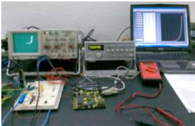
Figure 10, Hardware setup showing I-V on Oscilloscope and on the Laptop monitor using LabVIEW GUI Software.
