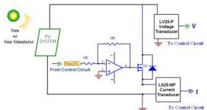
Figure 8, Illumination test circuit.
