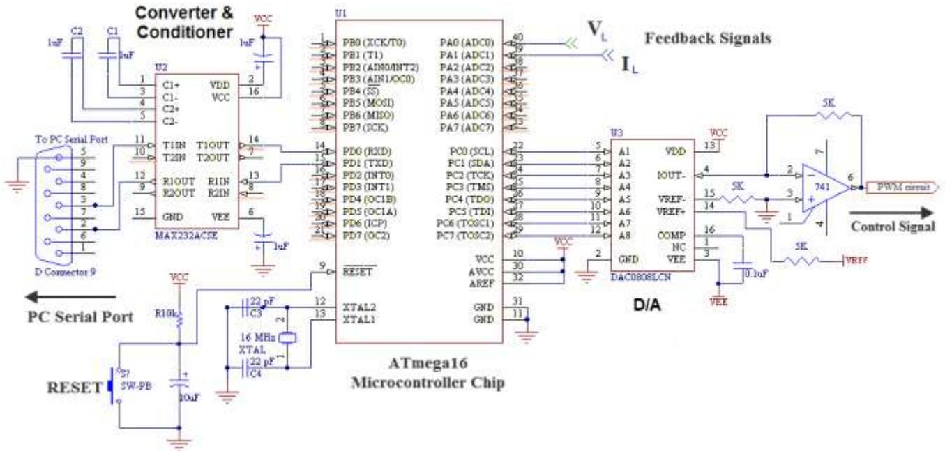
Figure 5, The microcontroller interfacing and measurement control circuit.
