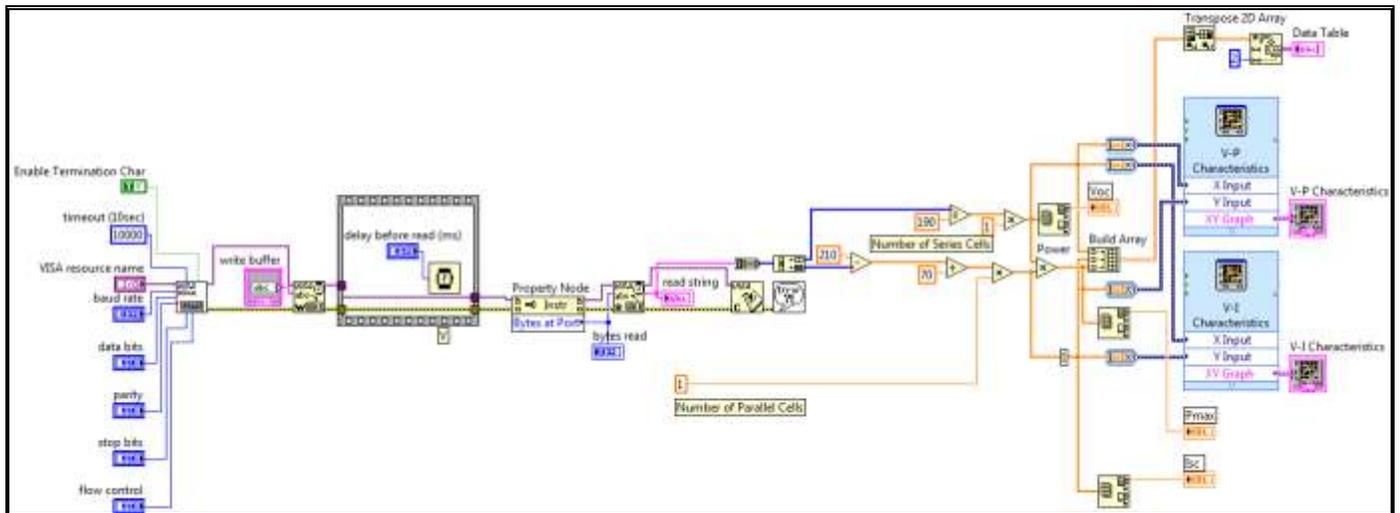
Figure 3, LabVIEW Serial Interface and I-V Curve Measurement Block Diagram
