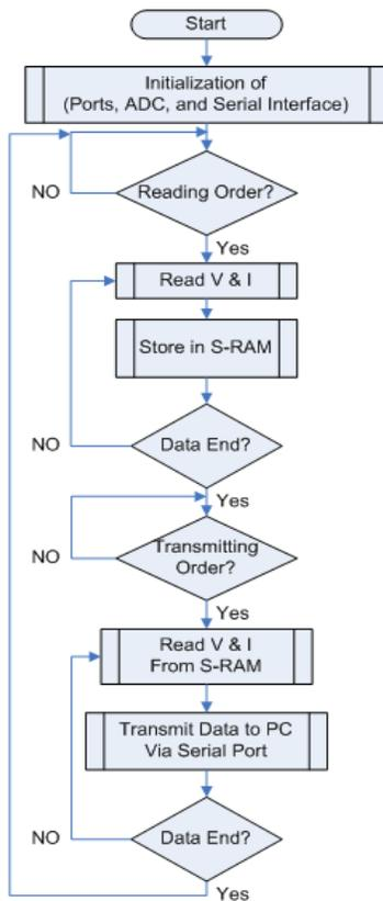
Figure 6, Microcontroller program flow chart.
