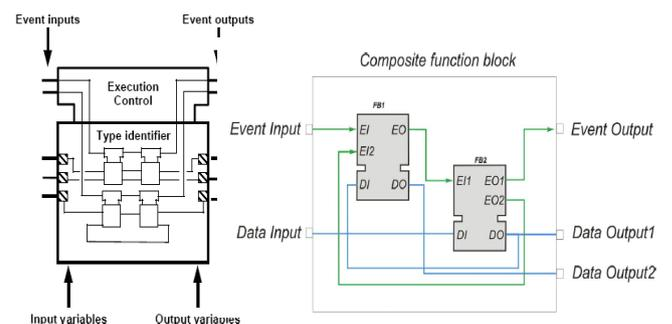
Fig. 6. Composite function block
