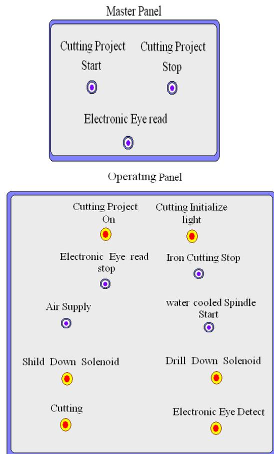
Fig. 11 Cutting Device Control Panels
