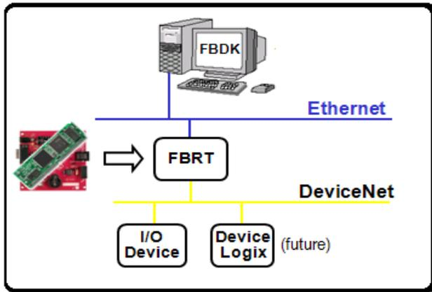
Fig. 9. FBDK and FBRT in creating IEC 61499 Function Blocks Environment
