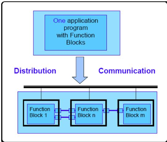
Fig. 1. IEC 61499 Distributed Function Blocks among Smart Field Devices
