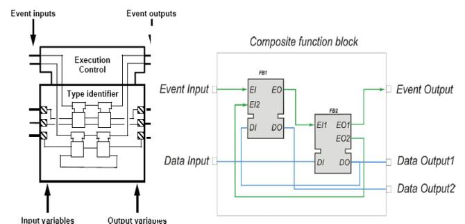
Fig. 6. Composite function block
