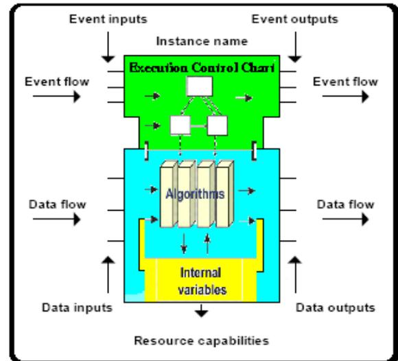
Fig. 5. IEC 61499 Function Block concept
