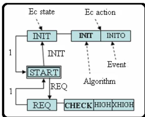
Fig. 8. IEC 61499 ECC of Function Block
