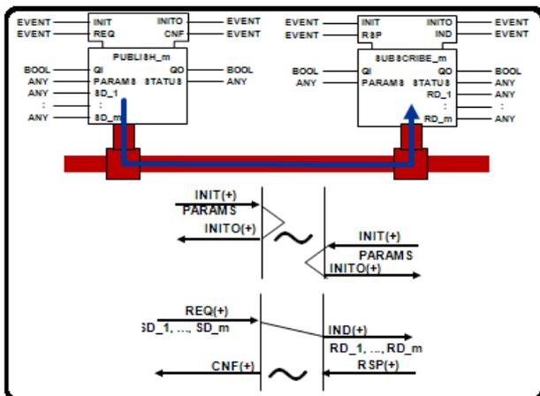
Fig. 10. Communication Service Interface using Publish subscribe Function Block
