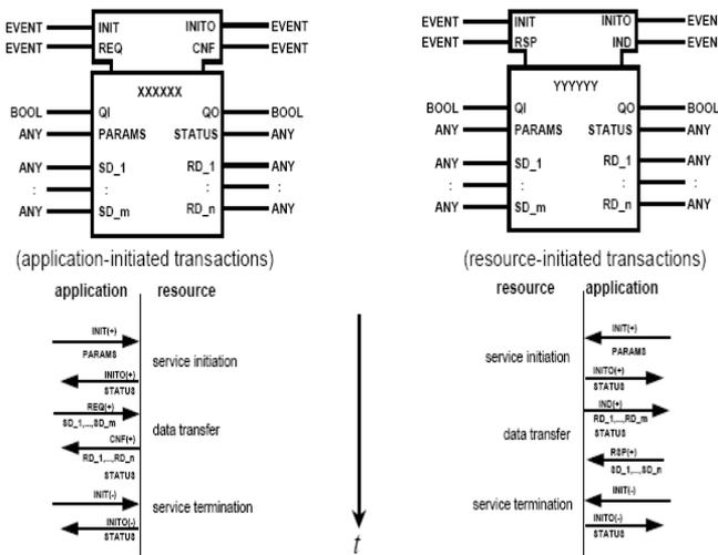
Fig. 7. Service Interface Function Block
