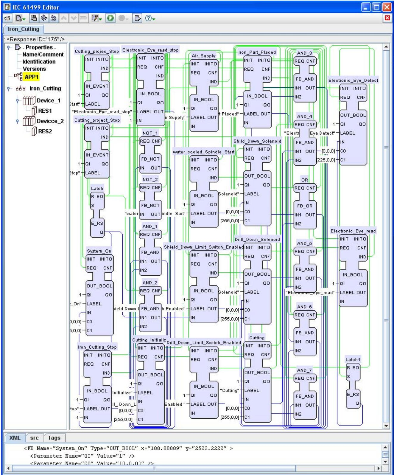
Fig. 15. IEC 61499 Iron Cutting Application
