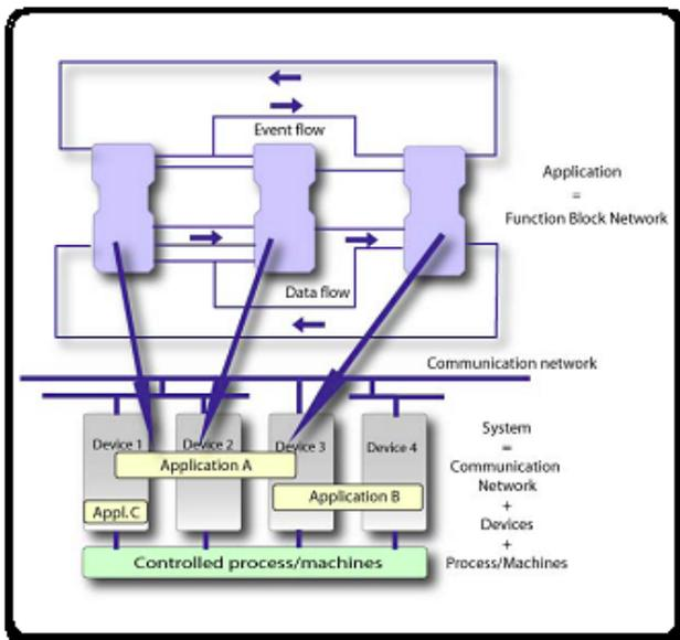
Fig. 4. Distributed System in IEC 61499
