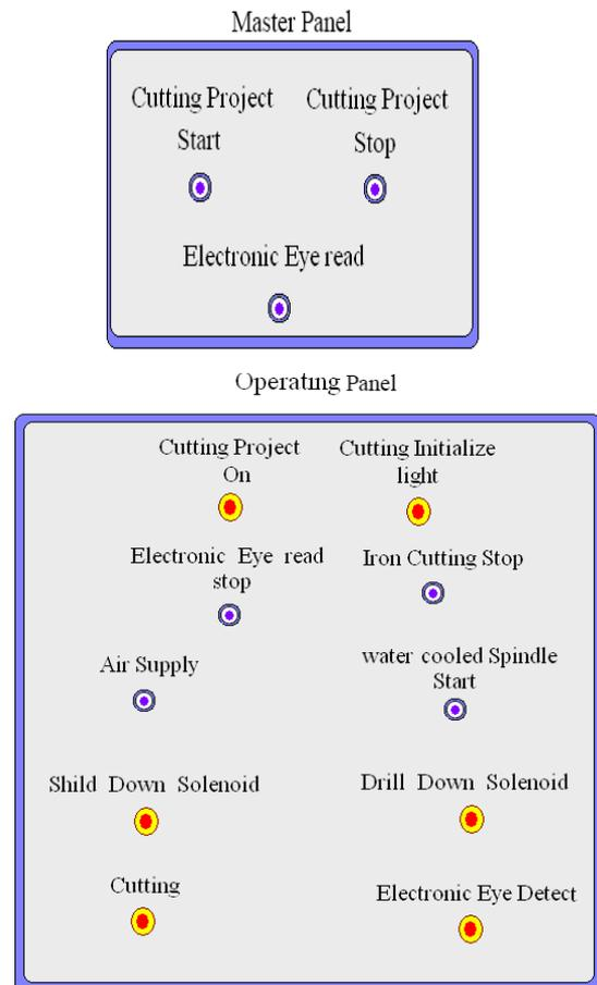
Fig. 11 Cutting Device Control Panels
