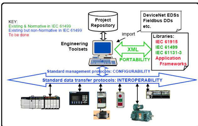
Fig. 2. Open Distributed System base on IEC 61499
