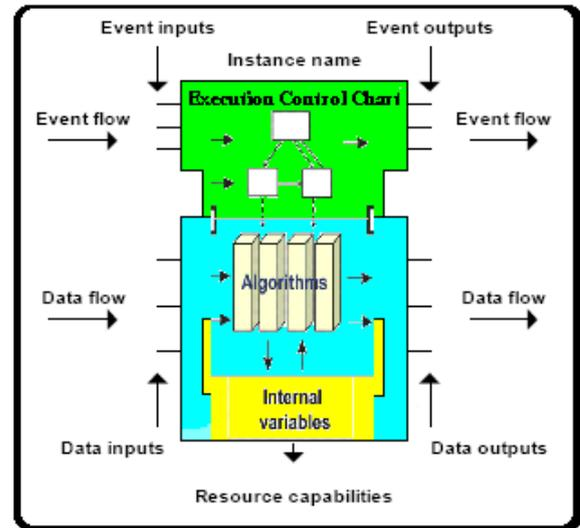
Fig. 5. IEC 61499 Function Block concept
