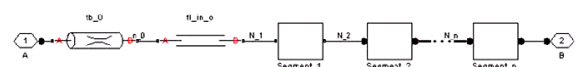
Fig.3 The mathematical model of the technological pipe using the SimHydraulics toolbox elements in Matlab
