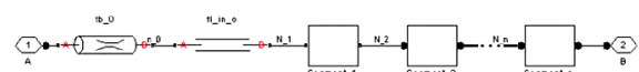
Fig.3 The mathematical model of the technological pipe using the SimHydraulics toolbox elements in Matlab
