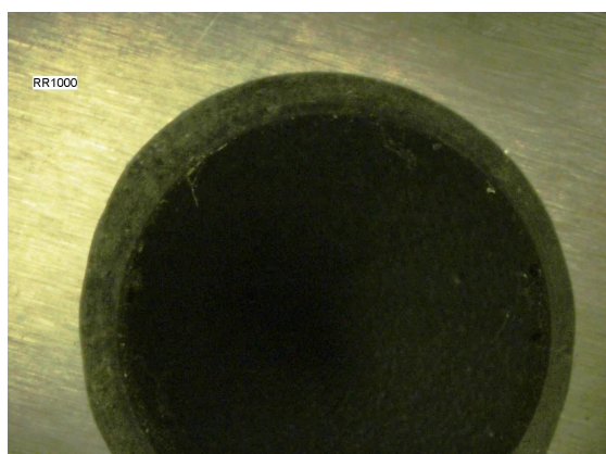
Fig. 16 A micrograph of deburred hole on RR1000 testpiece
