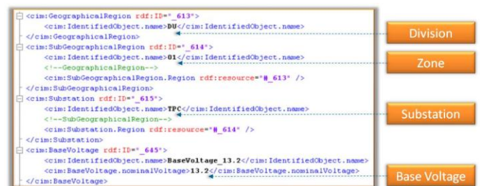
Fig. 12. Example of the Semantic Model (CIM based) for the On-Line Simulator.
