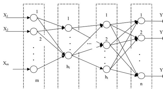
Figure 1 The generic architecture of a feedforward artificial neural network used in an environmental forecasting system.
