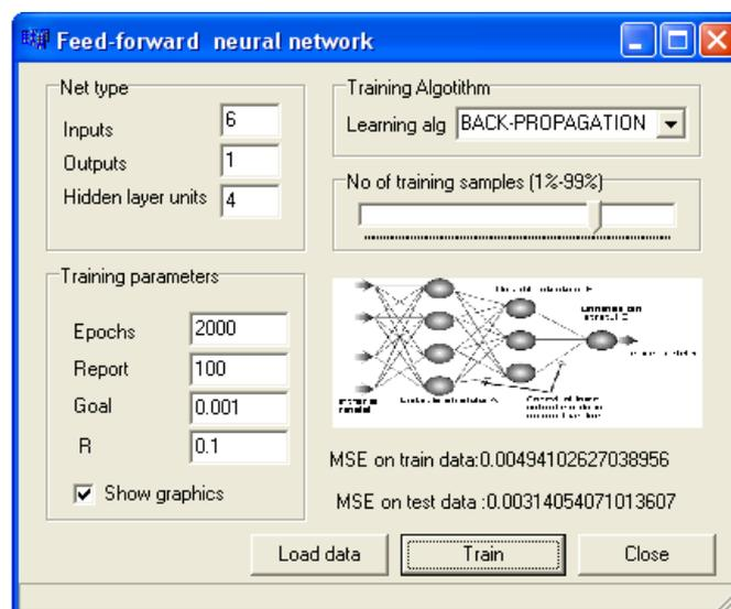
Figure 2 The interface of the air pollution forecasting system (based on the FANN library [5]).
