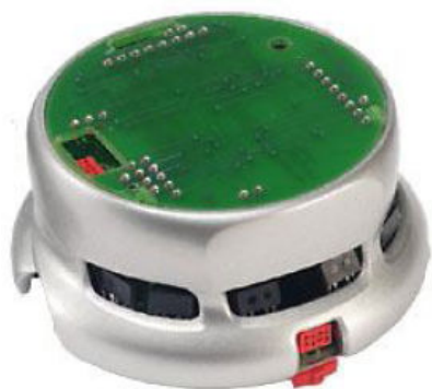
Fig.3 The Khepera II robot as a model of vacuum cleaner [7]
