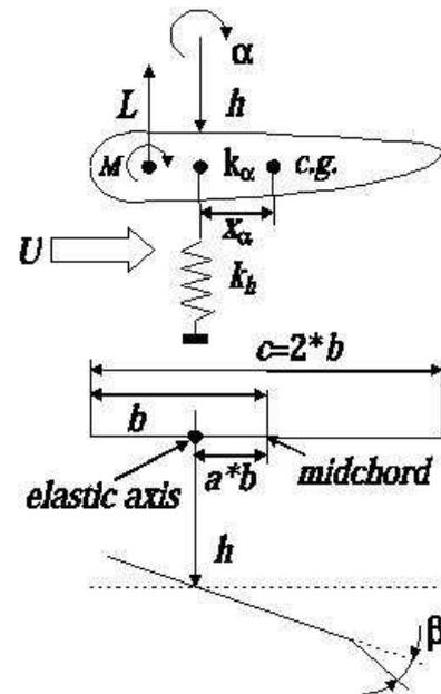
Figure 1. The aeroelastic wing section
