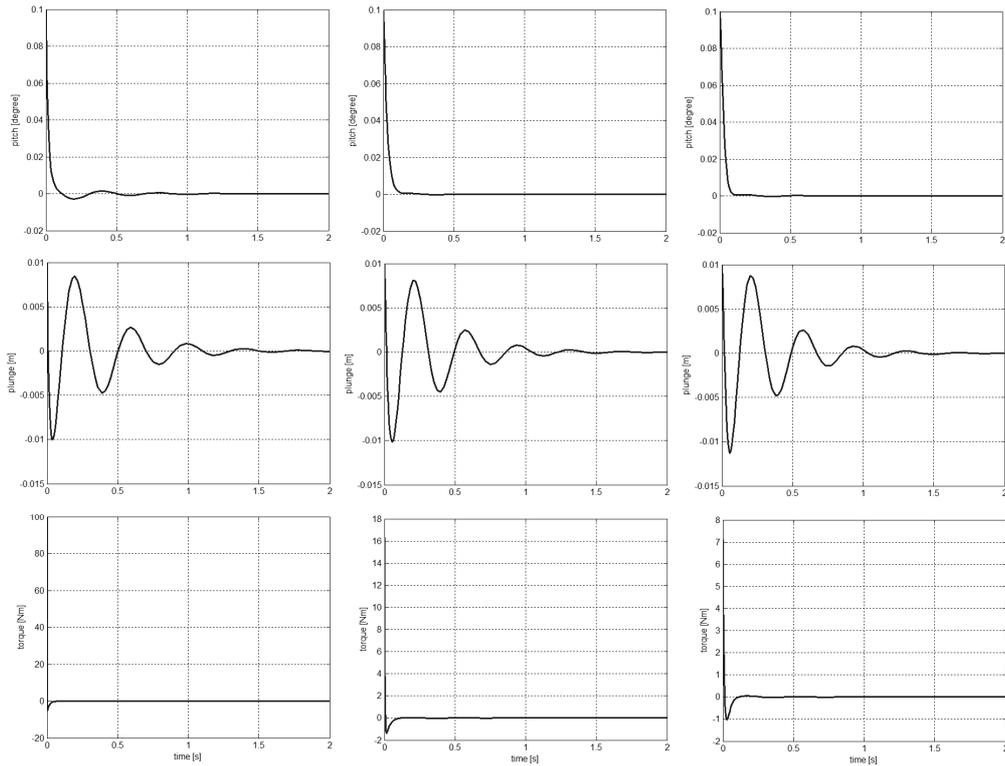
Figure 5. Time response of controller for  $U = 20$  m/s and  $a = -0.4$ , while  $Z=19$ ,  $Z=25$  and  $Z=30$ .
