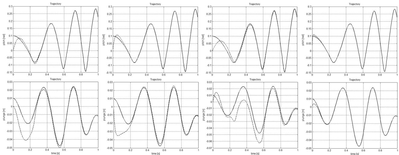
Figure 6.. Open loop simulation, while  $U=20$  m/s;  $Z=1$ (IRNO);  $Z=10$ ,  $Z=20$ ,  $Z=30$  (CNO)
