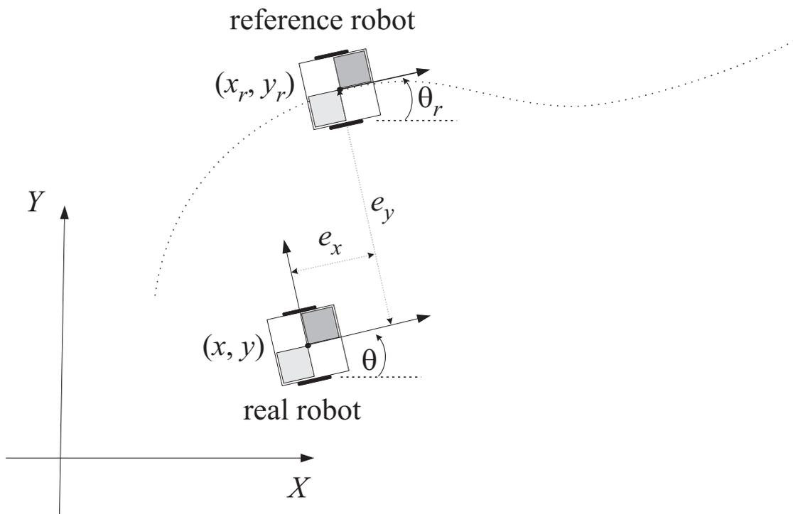
Figure 2: Illustration of the trajectory tracking control
