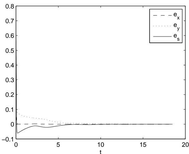
Figure 8: PDC-based control – time plots of the errors
