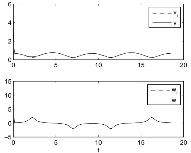
Figure 4: Lyapunov-based control – time plots of the velocities  $v(t)$  and  $w(t)$
