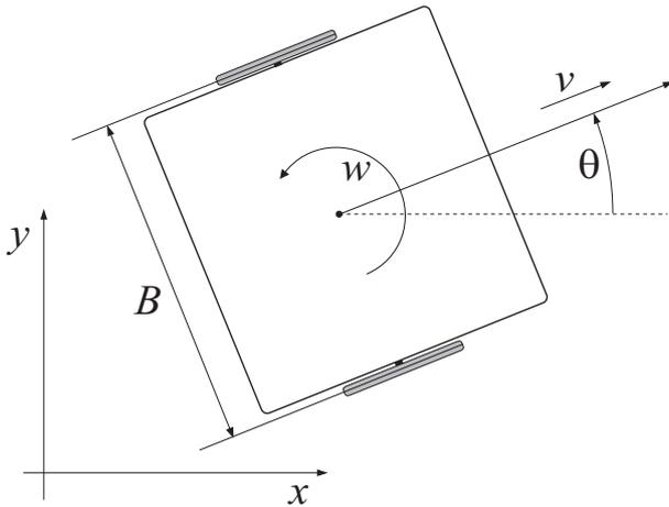
Figure 1: Two-wheeled, differentially driven mobile robot
