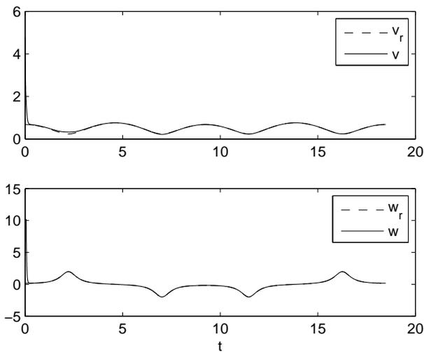
Figure 7: PDC-based control – time plots of the velocities  $v(t)$  and  $w(t)$
