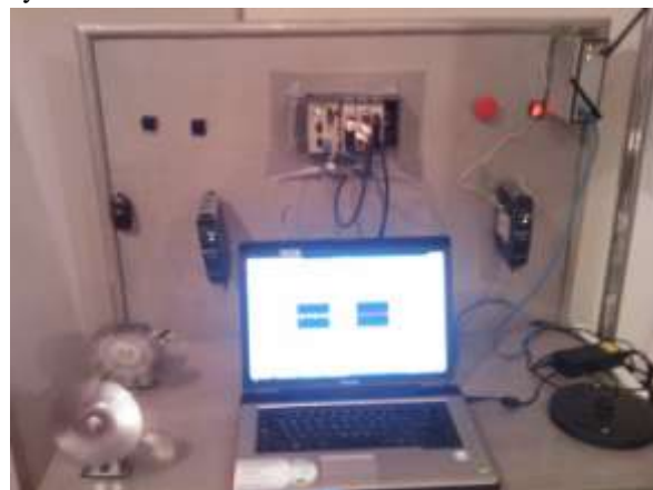
Fig 17, The Blue crossover cable is used to connect between the cRIO 9012 and the NI-WAP 3711.
