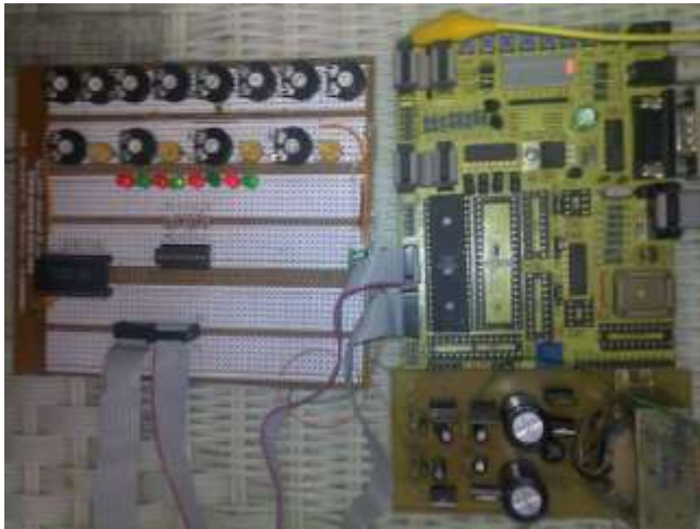
Fig 6, Emulator board and Computer Interfacing card.
