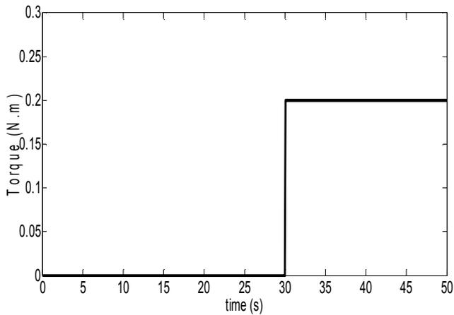
Fig.5 the plus step load acted upon the PMSM in simulation 2
