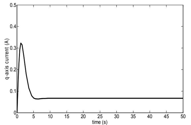
Fig. 3 the changing process of the current of the q-axis of the PMSM without load
