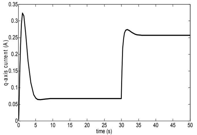
Fig.7 the changing process of the current of the q-axis of the PMSM with a plus step load
