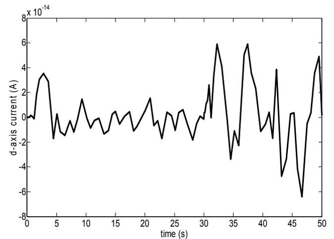
Fig. 8 the changing process of the current of the d-axis of the PMSM with a plus step load
