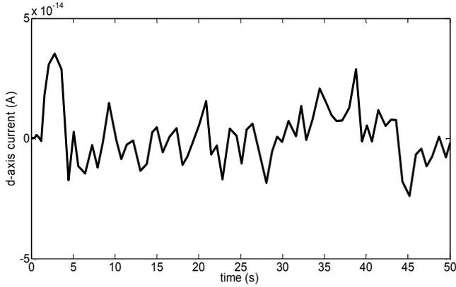
Fig. 4 the changing process of the current of the d-axis of the PMSM without load
