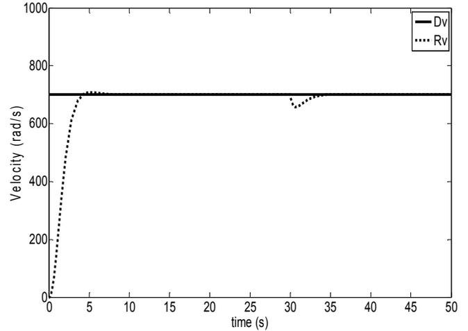
Fig.6 the process of the velocity tracing of the PMSM with a plus step load
