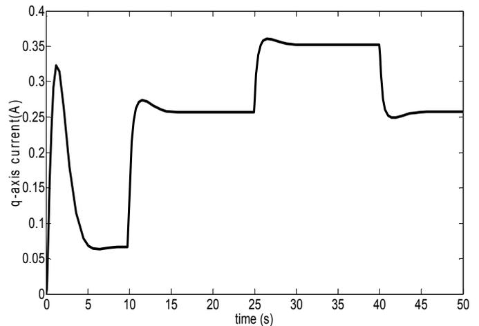
Fig. 11 the changing process of the current of the q-axis of the PMSM with a series of changing load
