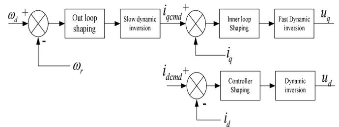
Fig. 1 the structure of the controller of the PMSM
