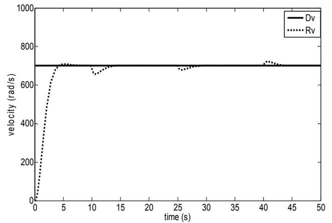
Fig. 10 the process of the velocity tracing of the PMSM with a series of changing load
