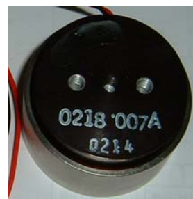
Fig. 2 Voice coil as the force actuator.
