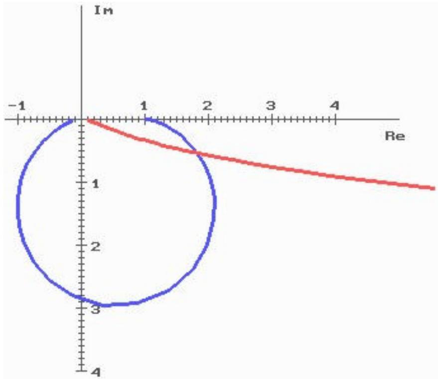
Fig.4 The hodograph of the open and closed speed adjustment system
