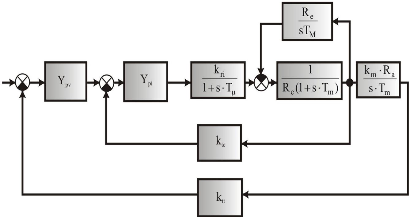
Fig.2 Speed regulation system structural schematics
