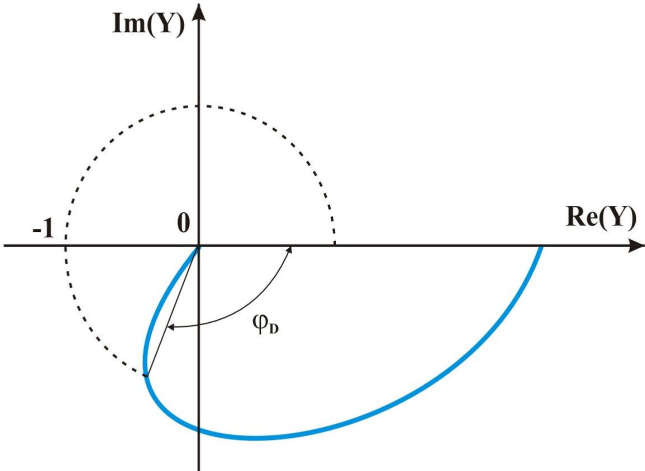
Fig.1 The place of transfer of a stable system
