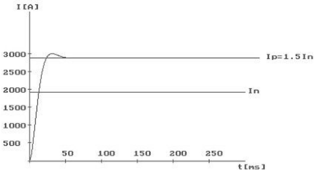
Fig.5 Current variations within the ignition of the main operation motor
