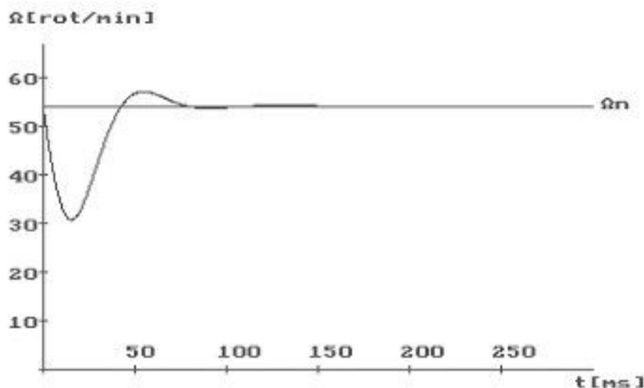
Fig.7 Speed variation diagram during a considerable load variation
