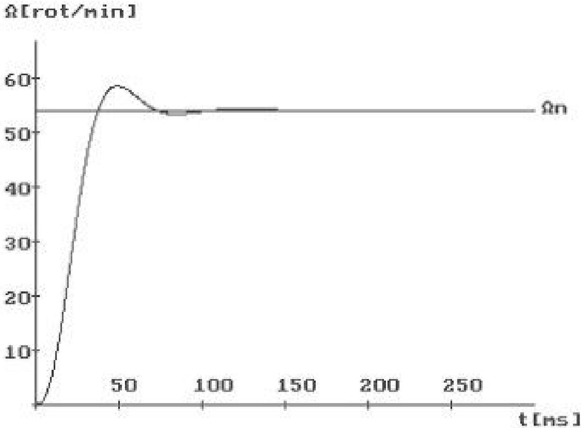
Fig.6 Ignition speed variation diagram
