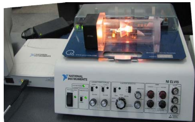
Figure 1. QNET HVAC process
