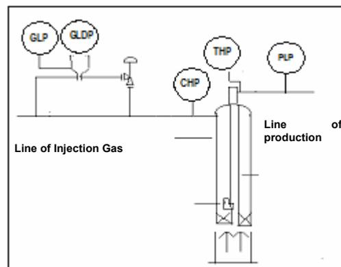
Fig. 8. Schematic design of the Well with the Extraction Gas Lift Method
