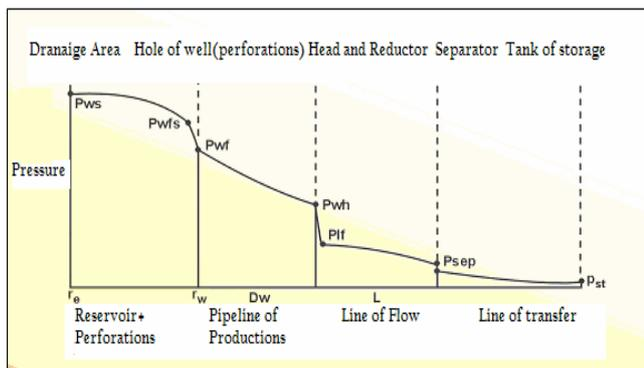
Fig. 5. The loss of energy in a Systems of Production
