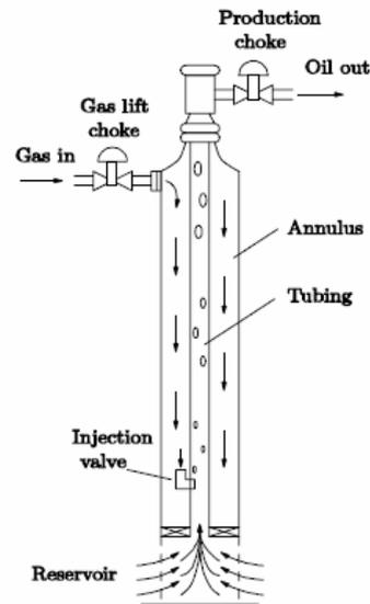
Fig. 6. The Artificial Gas Lift
