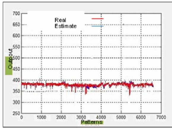
Fig. 16. Neo-Fuzzy Estimation of the Tubing Pressure
