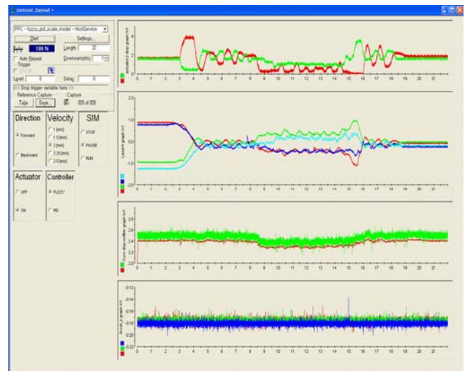
Fig.15 The experimental results (various sensor outputs): the actuator displacement signals, the four laser sensor output signals for relative displacements, the gyro sensor signals for measuring the bogie yaw angle, and the accelerometer output for a characteristic vibration of car-body, respectively.
