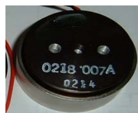
Fig. 2 Voice coil as the force actuator.
