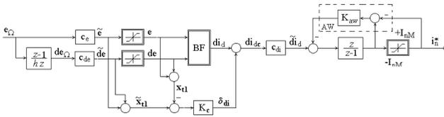
Fig. 15 The structure of the quasi fuzzy controller
