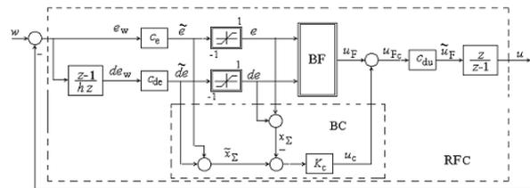
Fig. 10 Fuzzy controller with stability correction
