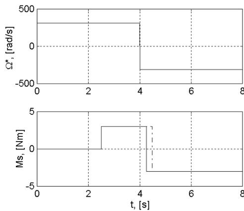
Fig. 20 Rotational speed reference  $\Omega^*$  and the load torque  $M_s$
