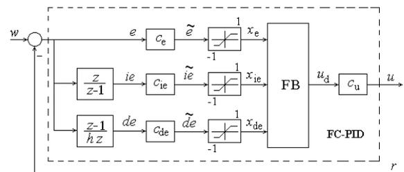
Fig. 13 The block diagram of PID fuzzy controller
