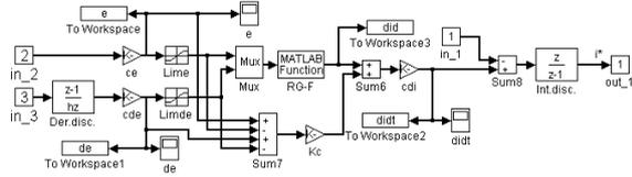
Fig.19 Simulink block diagram of the fuzzy controller
