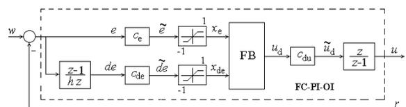
Fig. 8 The block diagram of the fuzzy PI controller
