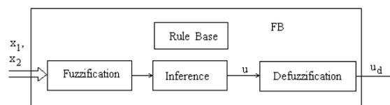
Fig. 2. The structure of the fuzzy block
