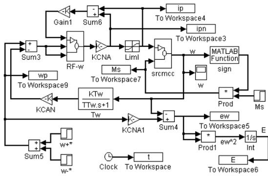
Fig. 18 Simulink block diagram of the speed fuzzy control system
