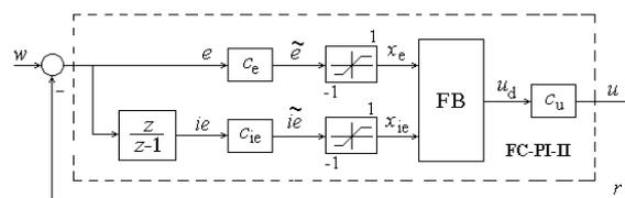
Fig. 11 The block diagram of the PI fuzzy controller with input integration
