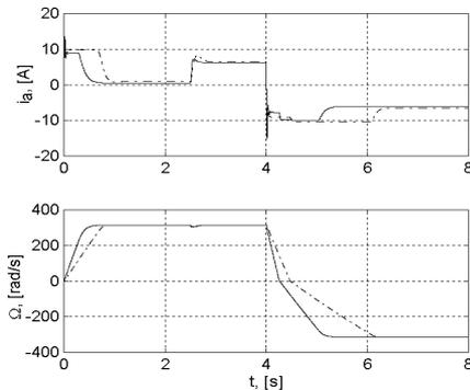
Fig. 24 Armature current  $i_a$  and the rotational speed  $\Omega$
