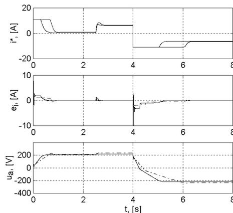
Fig. 23 The reference current  $i^*$ , the current error  $e_i$  the armature voltage  $u_a$
