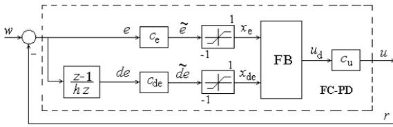
Fig. 12 The block diagram of the PD fuzzy controller
