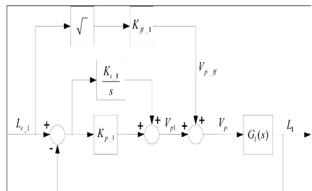
Fig.9 Tank 1 water level PI feedforward control loop
