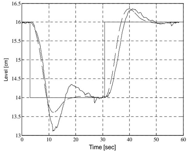
Fig.8 Step response system of L<sub>2</sub> level control
