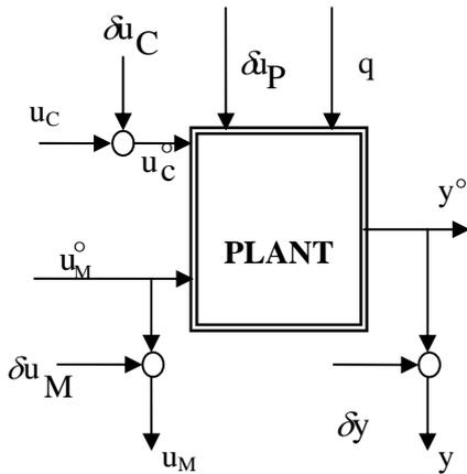
Fig.2 Additive disturbances and noises
