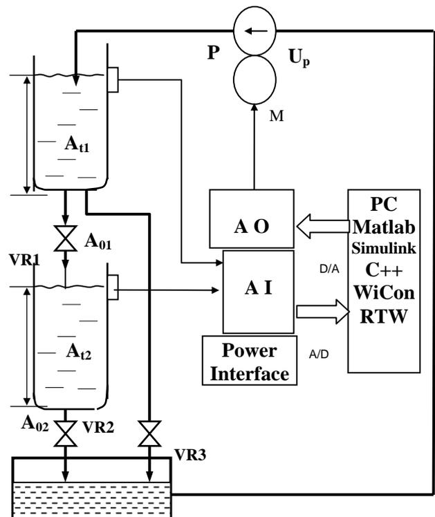
Fig.4 Technological diagram of the plant
