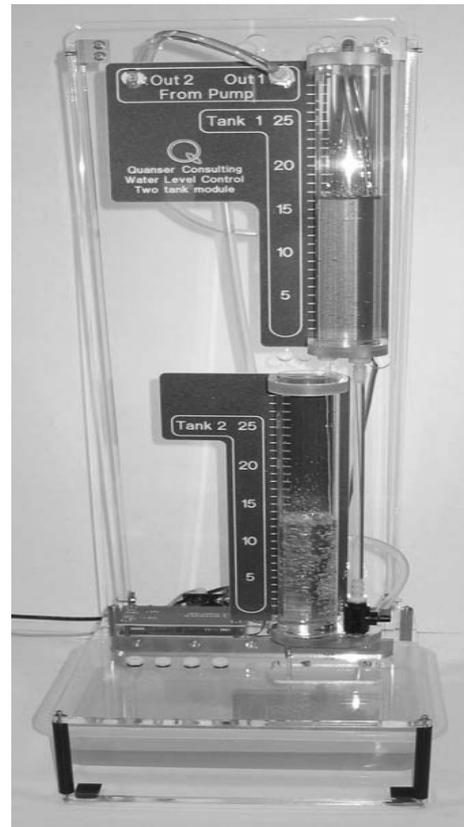
Fig.3 Didactical plant with coupled tanks
