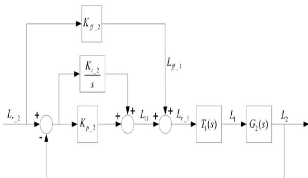
Fig.10 Tank 2 water level PI feedforward control loop
