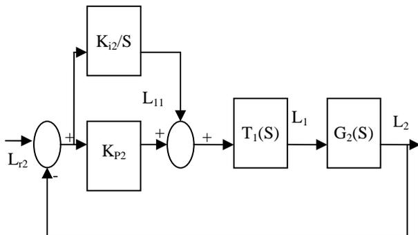
Fig.7 Tank 2 Water level PI control loop
