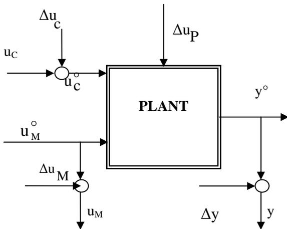
Fig.1 Additive faults
