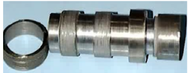
Fig. 8 Experiments damaged sample
