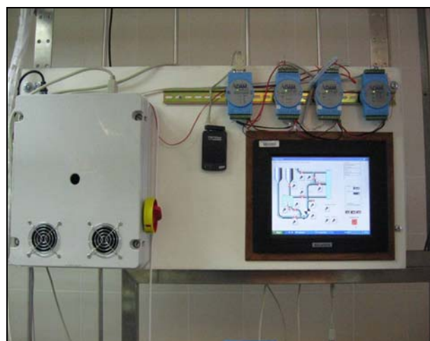
Fig. 21 Control board with panel PC and the control application running
