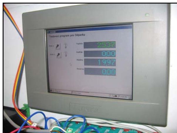
Fig. 10 Main window of a test program running on the TPC-650 panel PC.
