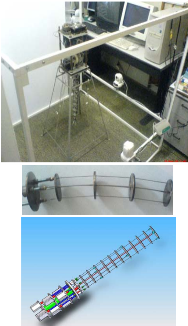
Fig. 1. a. Visual Control benchmark b. "Old" experimental segment c. CAD image of the tentacle design
