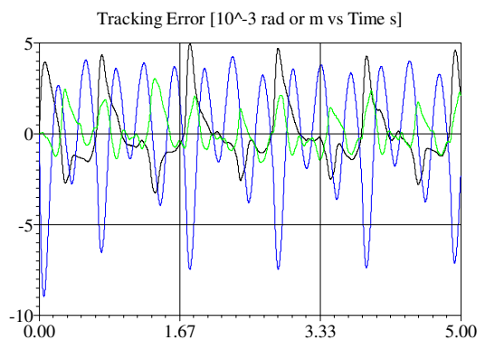
Fig. 11: Effects of imprecise dynamic model with friction and without disturbance forces: the Slotine-Li controller (the first two charts), the FPT/SDV-based controller (the second two charts)
