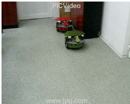
Fig. 16a The starting situation, the red mobile robot will follow the green robot
