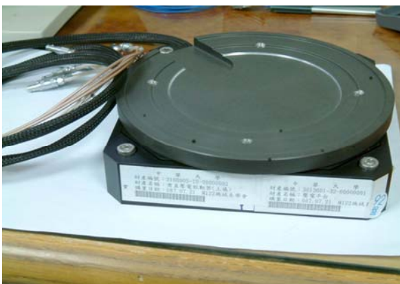
Fig.9 The piezo-stage and the sample holder.
