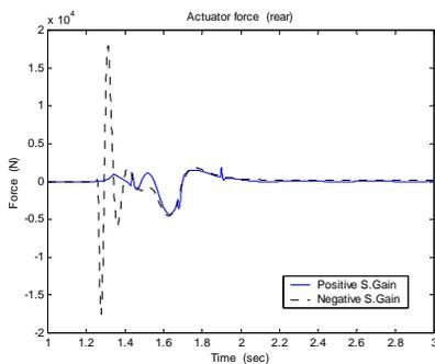
Fig. 25 Actuator force for varying the parameter  $\rho_{h_r}$
