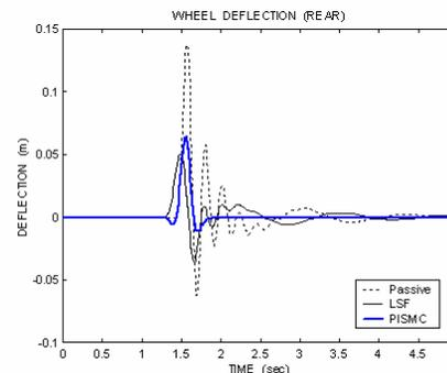
Fig. 7 Wheel deflection of the half car rear suspension (single bump)
