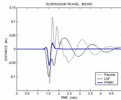
Fig. 5 Suspension travel of the half car rear suspension (single bump)
