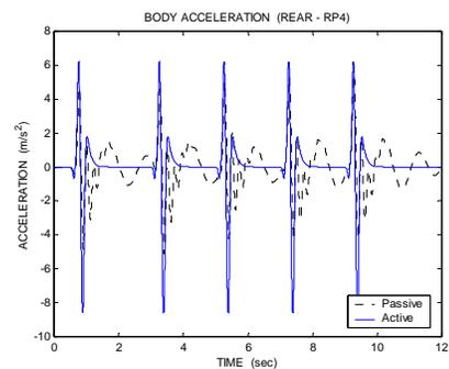
Fig. 15 Body acceleration of the half car rear suspension (multiple bumps)
