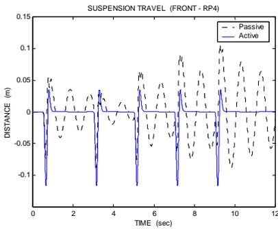
Fig. 10 Suspension travel of the half car front suspension (multiple bumps)
