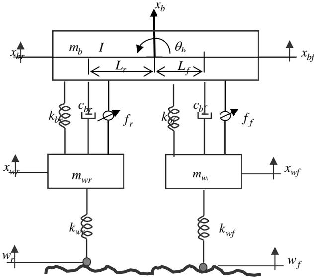
Fig. 1 The active suspension for the half car model
