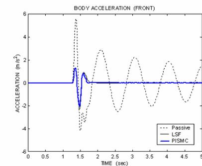
Fig. 8 Body acceleration of the half car front suspension (single bump)
