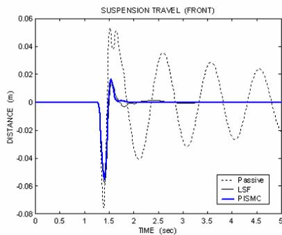
Fig. 4 Suspension travel of the half car front suspension (single bump)
