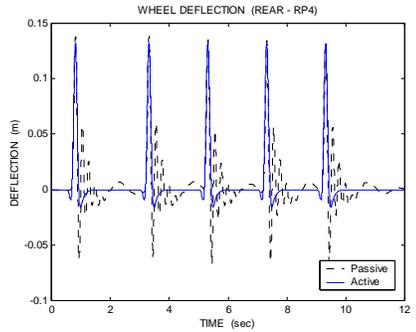
Fig. 13 Wheel deflection of the half car rear suspension (multiple bumps)
