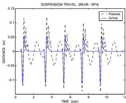
Fig. 11 Suspension travel of the half car rear suspension (multiple bumps)
