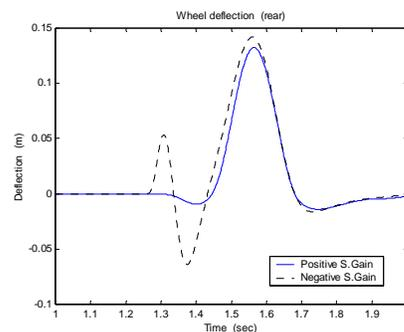
Fig. 21 Wheel deflection for varying the parameter  $\rho_{h_r}$
