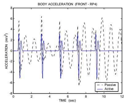
Fig. 14 Body acceleration of the half car front suspension (multiple bumps)
