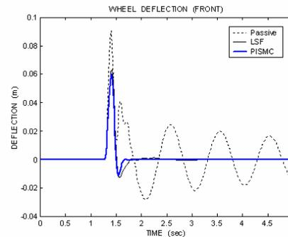
Fig. 6 Wheel deflection of the half car front suspension (single bump)
