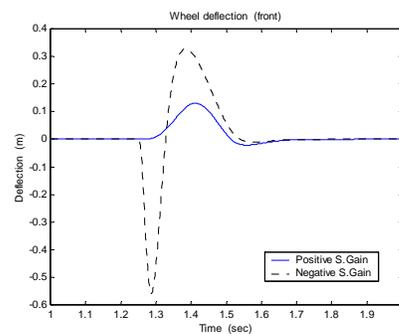
Fig. 20 Wheel deflection for varying the parameter  $\rho_{h_f}$
