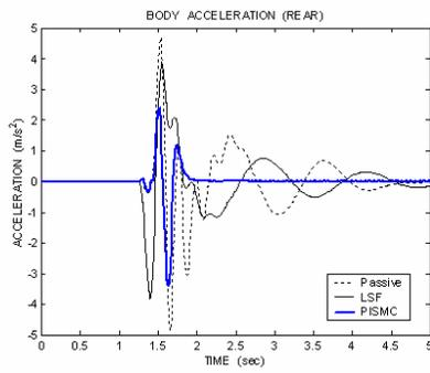
Fig. 9 Body acceleration of the half car rear suspension (single bump)
