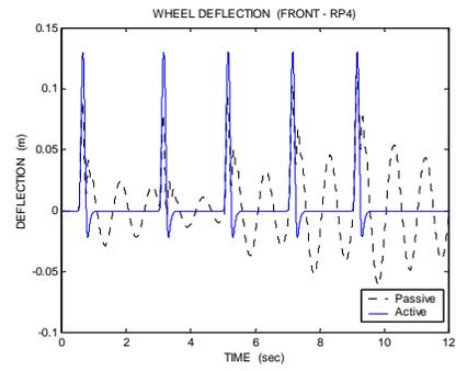
Fig. 12 Wheel deflection of the half car front suspension (multiple bumps)
