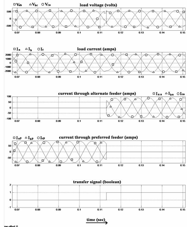
Fig.17: current through both feeders and load
