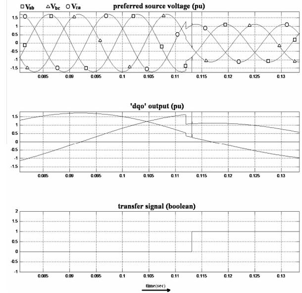
Fig. 16: Three phase under voltage in preferred source and transfer signal
