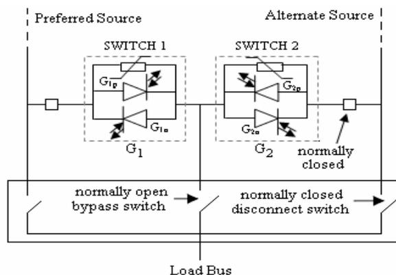
Fig.1: Basic structure of a single-phase STS
