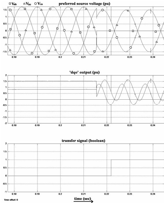
Fig.8: Occurrence and detection of fault
