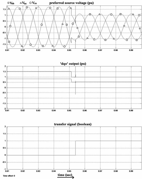
Fig.10: Three Phase Sag (35%) in Preferred Source Voltage
