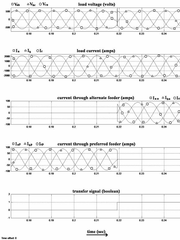
Fig. 14: Load current and transfer signal
