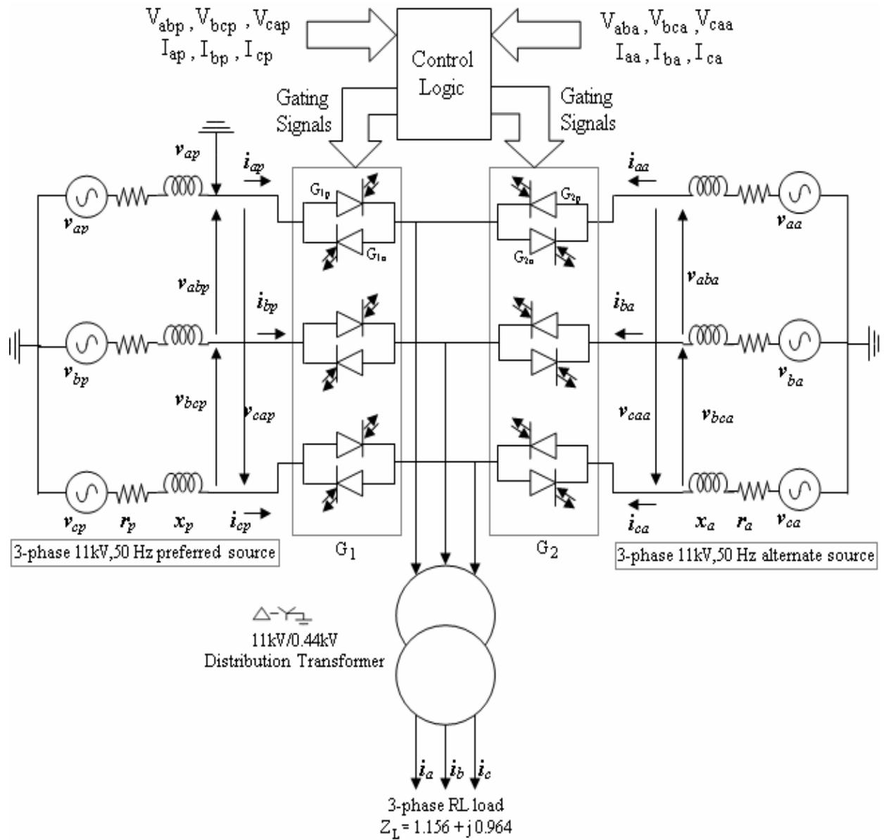
Fig. 2: Power Circuit of Three Phase STS System
