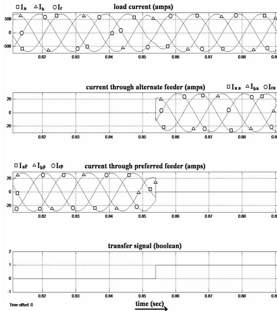
Fig.9: Detection of fault and load transfer
