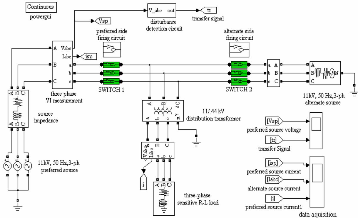
Fig. 5: Simulink model of three-phase STS system
