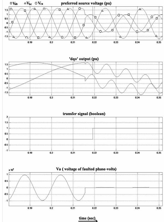
Fig.13: Source voltage and transfer signal
