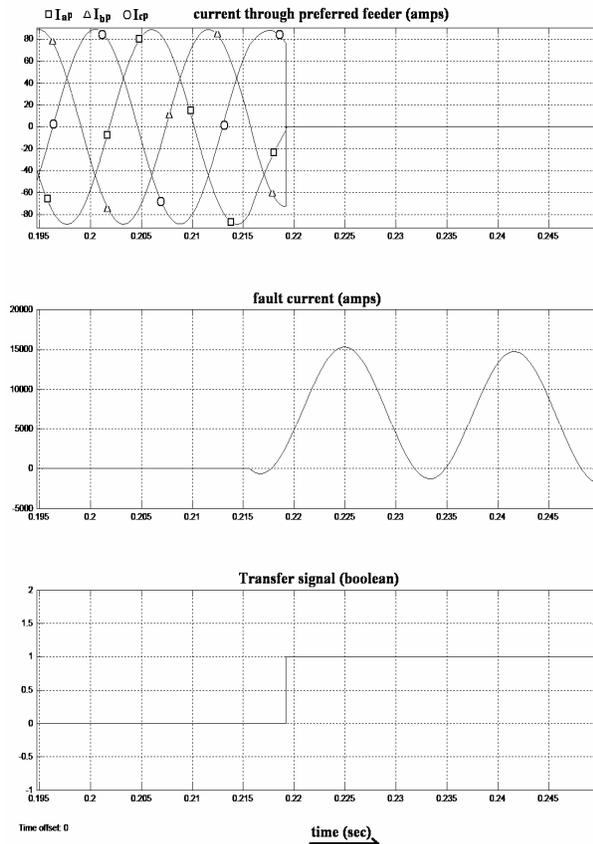
Fig. 15: Fault current and transfer signal
