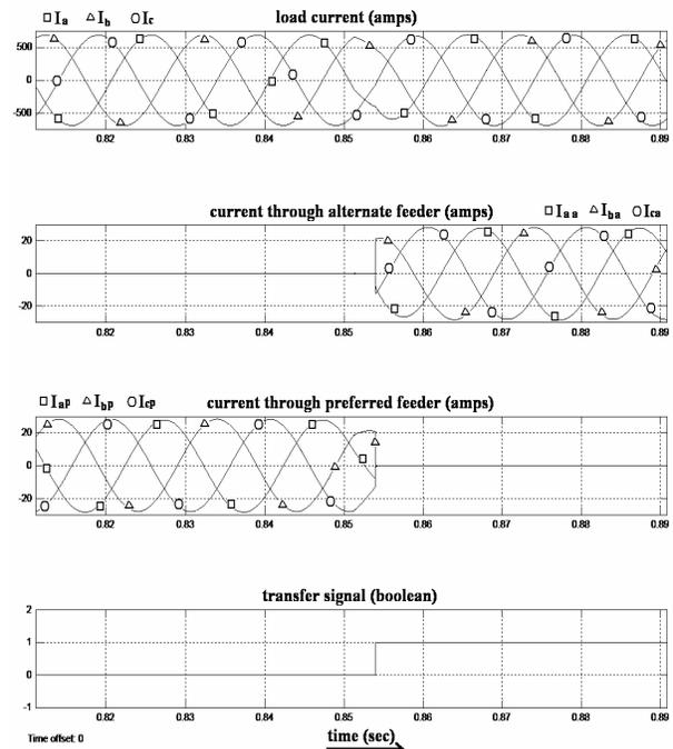
Fig.11: Current through both switches and load
