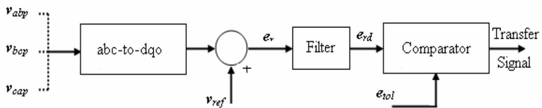
Fig. 3: Voltage Detection Scheme
