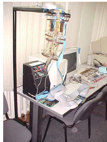
Fig. 23 Experimental model for a two module tentacle robotic structure
