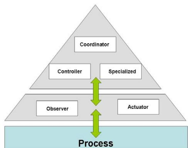
Fig. 1. Intelligent Distributed Control Based on Agents
