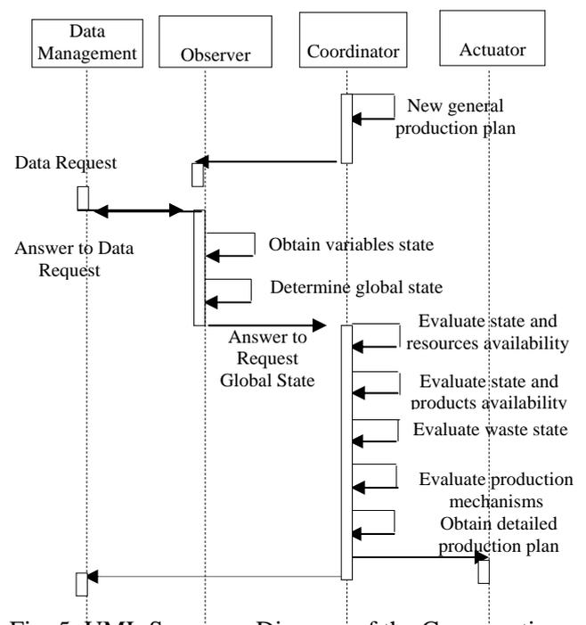
Fig. 5. UML Sequence Diagram of the Conversation “Design detailed plan”
