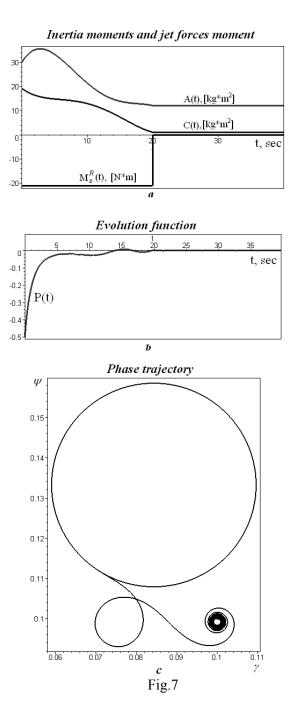
In considered case the magnitude of curvature becomes a constant after "shutdown" of jet moment and variability of the inertia moments. The phase trajectory form will pass to a circle of constant radius.
