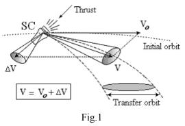
It is necessary to obtain the angular motion which ensures that SC's direct-axis (and the thrust vector) performs precessional motion with monotonously decreasing nutation angle. Thus the direct-axis travels inside an initial cone of nutation and the thrust vector naturally comes nearer to an axis of a precession which is a desired direction of transitional momentum output ("is focused" along a necessary direction).
