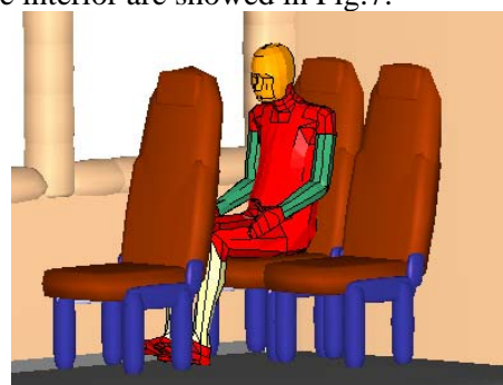
Fig.7 Occupant and vehicle interior model in MADYMO
