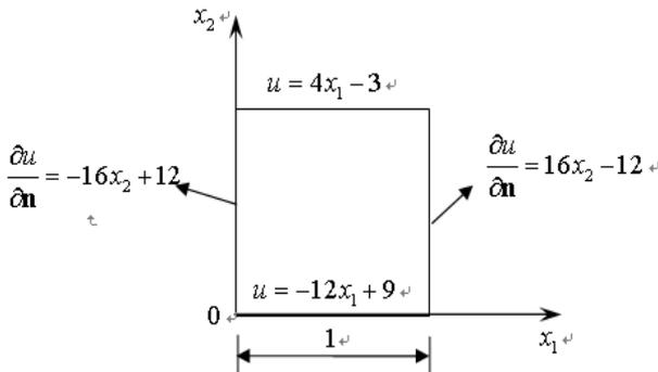
Fig. 2. Thermal transmission in a rectangular domain
