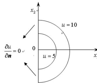
Fig. 5. Heat transmission in a thick cylinder.
