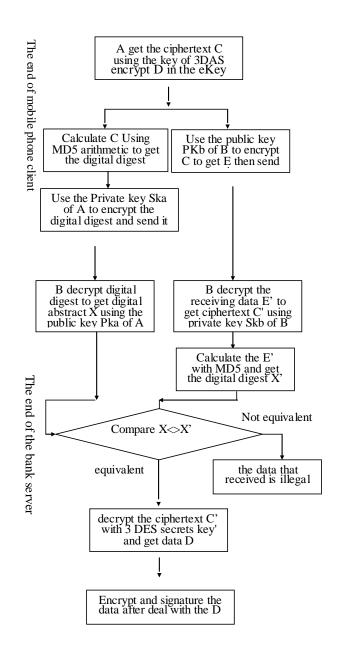
Fig. 2 Data Communication System process flowchart
