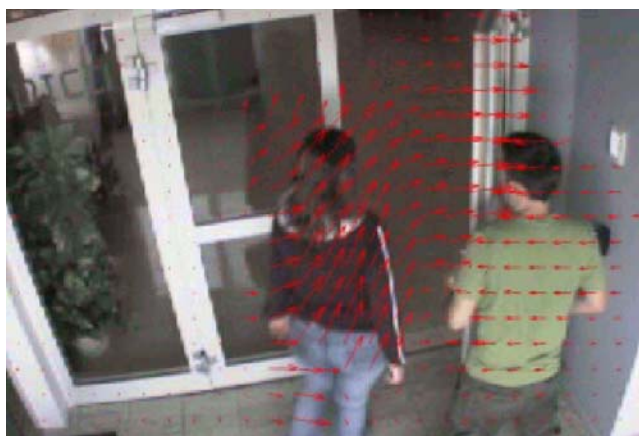
Fig. 7: The camera module recognizes parts of the video where some movement occurs and calculates the intensity of the movement. A new event video is classified based on similarity of other videos [18].
