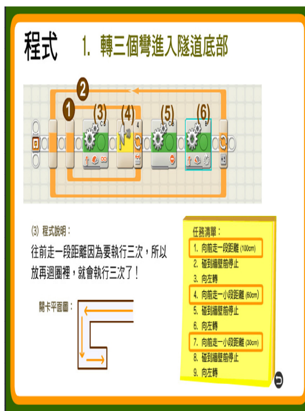
Fig. 9: The sample snapshot of LEGO MINDSTORMS NXT instructional material about how to define the parameters of servomotors.
