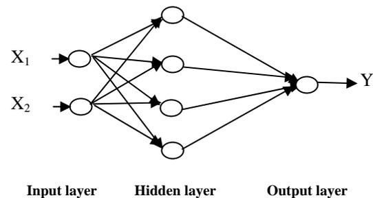
Figure 2. Structure of BP neural network Selected.
