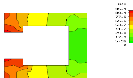
Fig. 5 Magnetic field distribution in Folded slot structure
