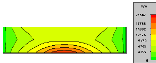
Fig.9 Electric field distribution in Folded slot structure.
