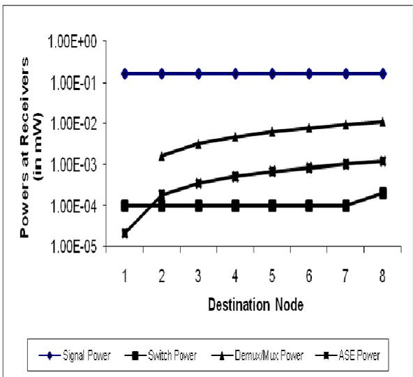
Fig. 4 Progress of a tagged call from Node 0 to Node 8 in a bidirectional ring network. The figure shows the signal, switch crosstalk, demux/mux crosstalk and ASE noise powers at the receivers of the intermediate nodes and the destination node
