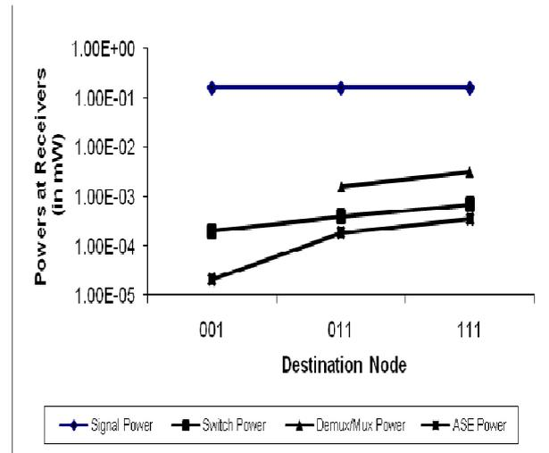
Fig. 5 Progress of a tagged call from Node 000 to Node 111 in a hypercube network. The figure shows the signal, switch crosstalk, demux/mux crosstalk and ASE noise powers at the receivers of the intermediate nodes and the destination node
