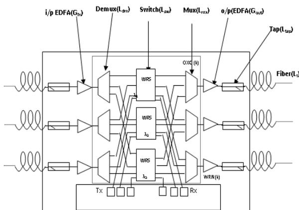
Fig. 1 Components in a wavelength routing node (WRN) [8]
