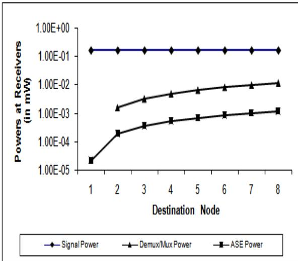
Fig. 3 Progress of a tagged call from Node 0 to Node 8 in a linear array network. The figure shows the signal, demux/mux crosstalk and ASE noise powers at the receivers of the intermediate nodes and the destination node
