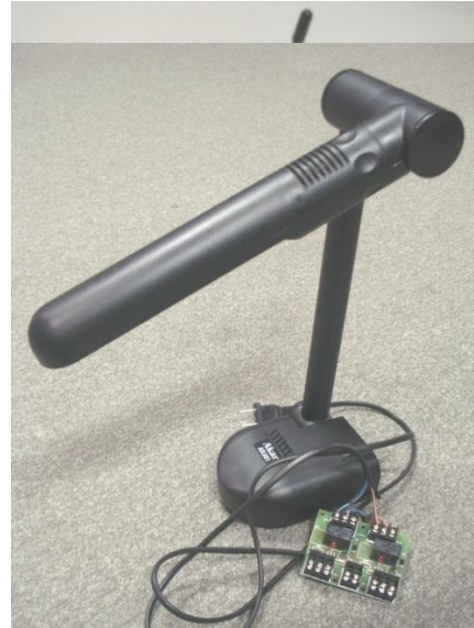
Figure 6: Lamp with relay driver
