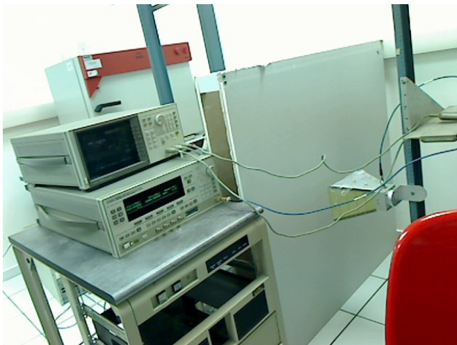
Fig. 13. Measurement of a triple layer gypsum wall. The gypsum layers are d=10 cm apart the k vector angle with respect to the normal is 0^0 .
