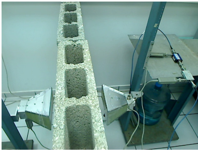
Fig. 19. Measurement of reflection and transmission from a concrete wall. The dimensions of each block in the wall are given in figure 20 below, the antennas are 8 cm from the wall and the k vector angle with respect to the normal is 0°.
