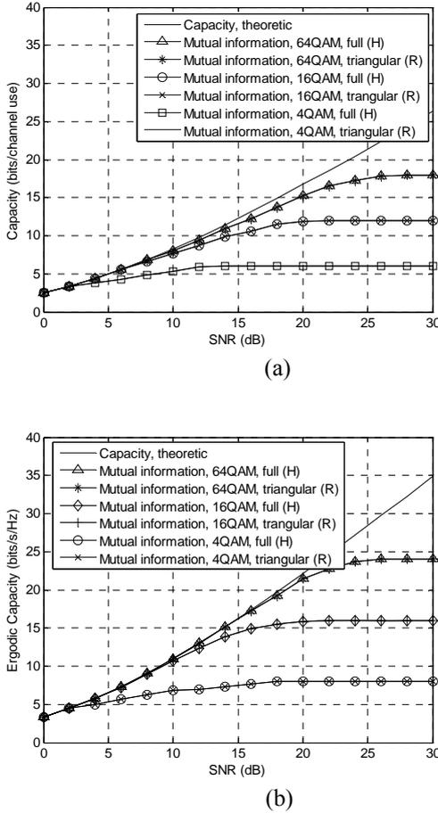
**Fig. 8. Ergodic capacity versus SNR performance for various modulation orders employing (a)  $N = 3, M = 3$ , (b)  $N = 4$  and  $M = 4$ .**
