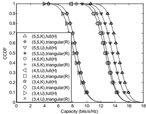
Fig. 7. CCDF versus capacity for various antenna configurations at SNR = 10 dB.
