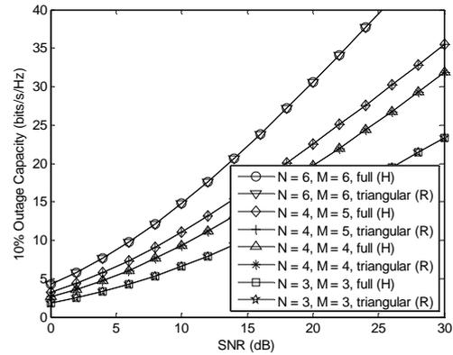
Fig. 6. Outage capacity versus SNR performance for various antenna configurations.
