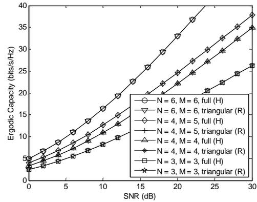
Fig. 5. Ergodic capacity versus SNR performance for various antenna configurations (s denotes second).
