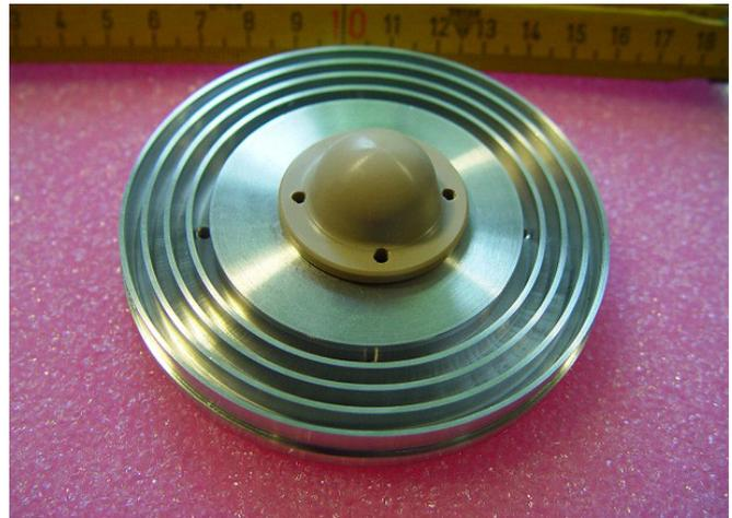
Fig.8 Ku band antenna with 4 chocherings.
